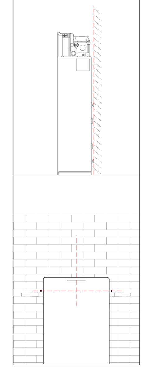
e. Remove the handlebars and take out the mounting lugs and align them with the holes on the both sides. Insert the M6 screws and tighten the screws with a torque of 3 N·m.
