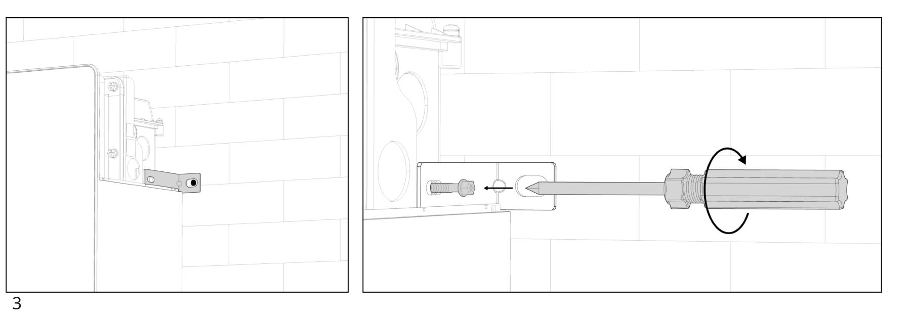
d. Take out the mounting plate and align it with the holes. Insert and tighten the screws with a torque of 9–14 N·m.
