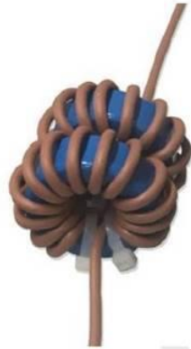
Figure 6: Toroid Rings Fitted on a Small Core Phase Cable
