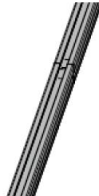
Fig 4.2.2C: Rails secured together via Proline joiner
