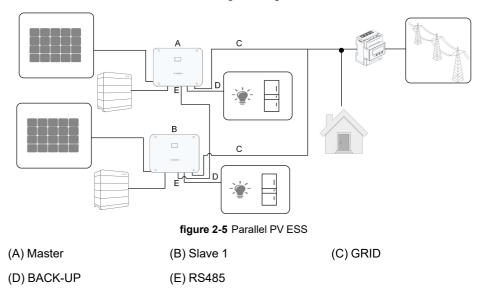
Only the hybrid GRID terminals can be connected in parallel, the LOAD terminals and the battery terminals cannot be connected together. The backup loads of each inverter should not exceed its nominal power.
