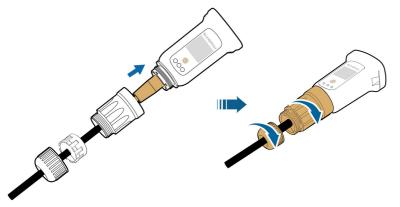
step 6 Remove the waterproof lid from the WLAN terminal and install WiNet-S.
