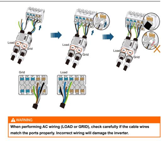
step 7 Ensure that the wires are securely in place by slightly pulling them. Tighten the swivel nut to the housing.
