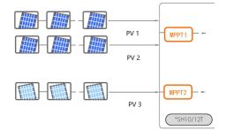
For SH15T/20/25T, each pair of PV terminals is corresponding to an independent PV string. PV input PV1, PV2 connect to MPPT1, PV3, PV4 connect to MPPT2 and PV5 connect to MPPT3. For the best use of PV power, PV1 and PV2, PV3 and PV4 should be the same in PV string structure, including the type, number, tilt, and orientation of the PV modules.
