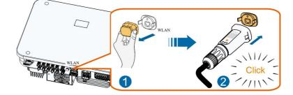
step 7 Slightly shake it by hand to determine whether it is installed firmly.
