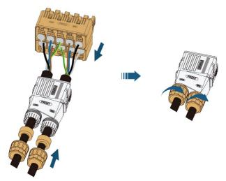
step 8 Insert the AC connector into the **GRID and LOAD** terminal on the inverter until there is an audible sound.
