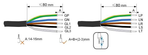
The color of the cable cores in the figure is for reference only, and cables or cable cores selected must meet local standards.
