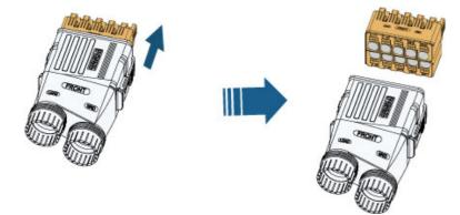
step 3 Thread the AC cable of appropriate length through the swivel nut and the housing.
