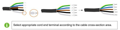
step 6 When wiring, the five wires (LOAD or GRID) should be correctly positioned according to the marks and inserted into the terminal at the same time. After finishing wiring, make sure the cold-pressed terminal does not protrude from the outside surface of the AC terminal.
