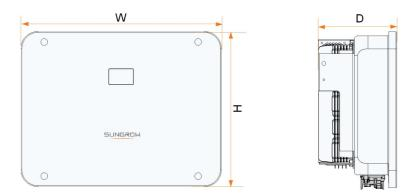
figure 2-2 Dimensions of the Inverter
