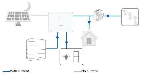
During night, when the battery is empty, it will enter into standby mode. In this case, the grid will supply all power for loads.
