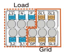
There are two different markings for the AC wiring terminals, one is the combination of GR, GS, GT, LR, LS, and LT, and the other is the combination of GL1, GL2, GL3, L1, L2, and L3 (as shown above). The actual product should take precedence. For the GRID terminals, GL1, GL2, and GL3 indicate live wires, GN indicates N wire, and GP indicates ground wire.
