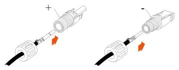
step 4 Check for polarity correctness.
