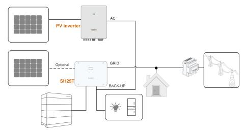
Load Terminal to Retrofit the Existing PV System
