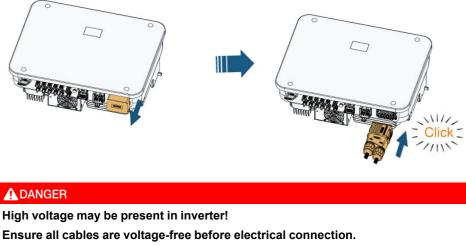
Do not connect the AC circuit breaker until all inverter electrical connections are completed.
