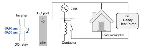
figure 8-24 DO Operation in Timing Mode
