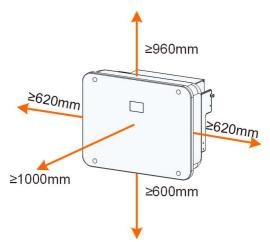
In case of multiple inverters, reserve specific clearance between the inverters.
