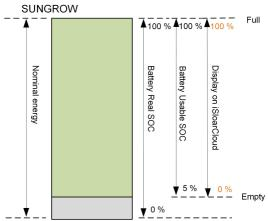
The SOC limits of Li-ion batteries can be modified via the iSolarCloud App by qualified personnel.
