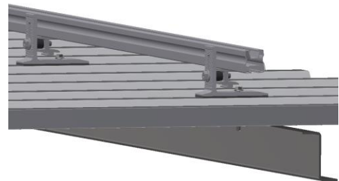
Fig 4.2.3B: Rail attachment to fasteners
