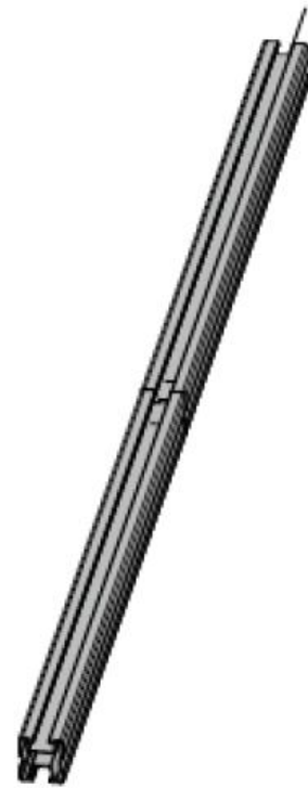
Fig 4.2.2C: Rails secured together via Proline joiner
