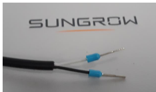
Picture 9 – The correct bootlace crimps
