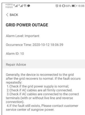
figure 7-9 Detailed Fault Alarm Information
