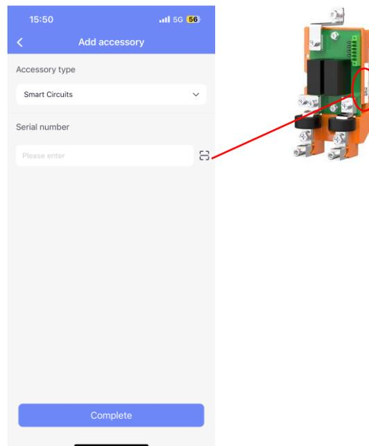
Step 6. Repeat the previous steps to bind the generator module. The QR code locations for the Generator Module is shown below.
