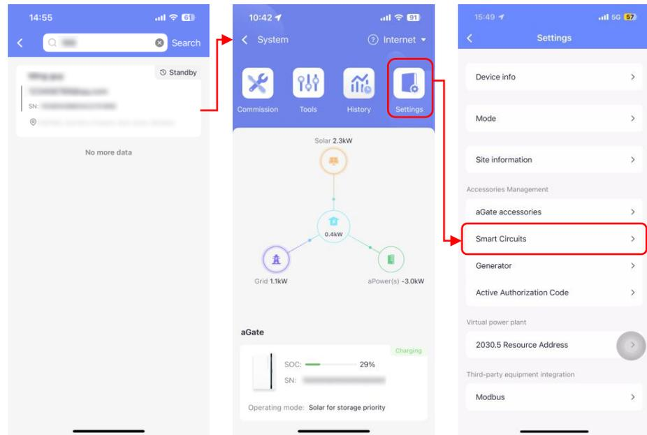
Step 2. If the switch is highlighted, it indicates that the corresponding circuit is operating. If the switch is dark, it indicates that the circuit is disabled. Click the button for the corresponding load module to enable or disable a circuit, then click to set the dedicated power plan for that circuit.
