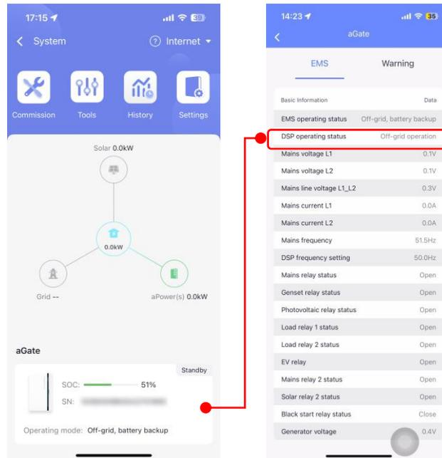
Step 5. Turn on the grid breaker and the FHP will switch to on-grid operations within 5 minutes. After the FHP is connected to the grid, click **Tools** and enable the **Go Off-Grid** button.
