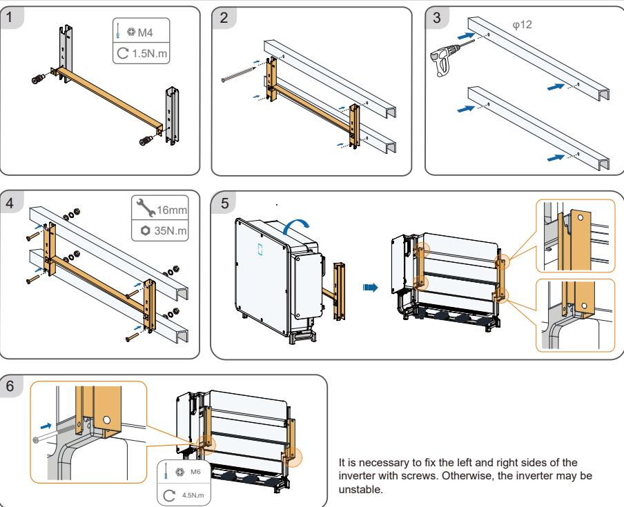
It is necessary to fix the left and right sides of the inverter with screws. Otherwise, the inverter may be unstable.
