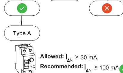
Allowed:  $I_{AN} \geq 30 \text{ mA}$
