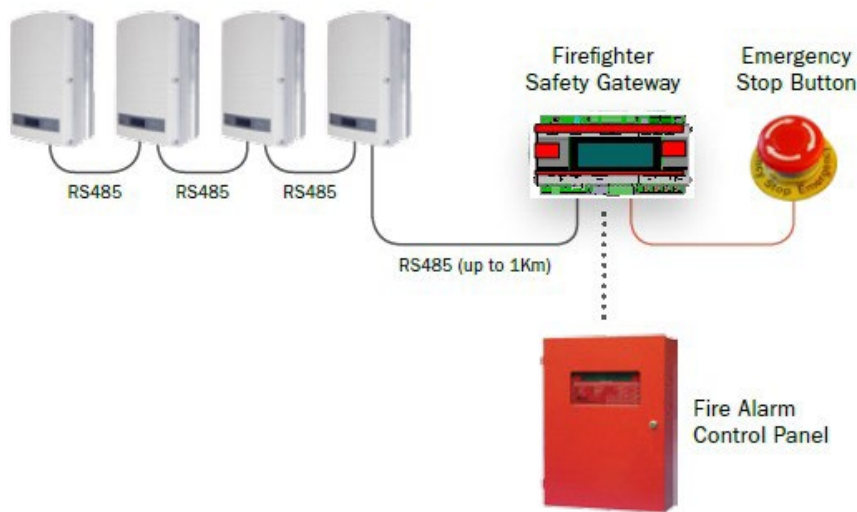
Figure 2: Example of SolarEdge firefighter gateway connections
