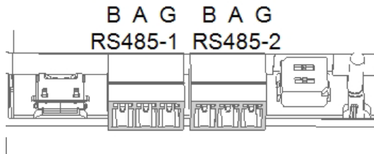
Figure 8: RS485 connectors and termination switches
