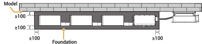
In this scenario, when the installation height of the inverter/PCS is lower than that of the Main Stack, to avoid derating due to heat exchange between the inverter/PCS and BAT during operation, a metal separator must be added between them. The metal separator must meet load-bearing requirements.
