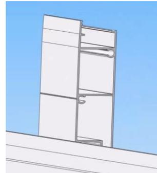
Fig 4.2.3B: Adding Pro Heightening Element to FixZ Rail
