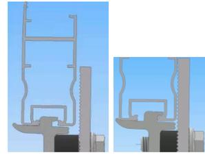
Fig 4.2.3A: FixZ Rail positioned to secure to fasteners
