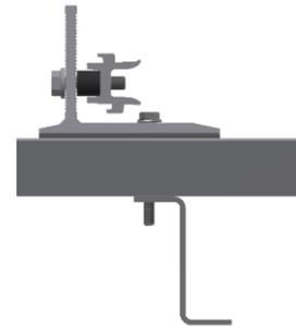
Fig 4.1.3: Rapid<sup>2+</sup> Pro SMLs being attached to using universal screw
