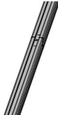
Fig 4.2.2C: Rails secured together via Proline joiner
