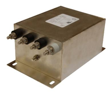
In commercial applications, the LCF-250-PC Line Filter, manufactured by Radius Power, separates power line communication domains across the Enphase Microinverter™ installation when multiple Envoys are located on a single utility transformer or when site loads generate electrical noise that disrupt communications. The integrated phase coupler allows microinverter power line communication to bridge phases.
