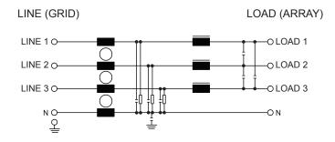
Connect both the Enphase  $Envoy^{\mathbb{M}}$  and Enphase Microinverters on the array or load side of the filter, and wire the utility feed to the line side of the filter.
