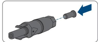
12. Insert the DC connectors with sealing plugs into the corresponding DC inputs on the inverter.
