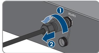
4. Screw the protective cap onto the RS485 jack.
