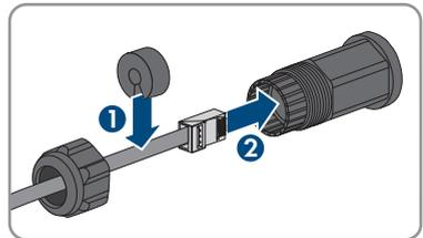
5. Press the cable support sleeve into the threaded sleeve.
