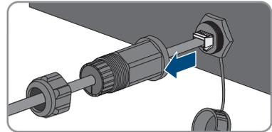
8. Take the cable support sleeve out of the threaded sleeve and remove the network cable from the cable support sleeve.
