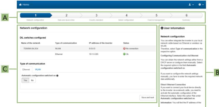
Figure 14: Layout of the installation assistant (example)
