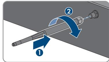
4. Pull on the WLAN antenna to ensure that the WLAN antenna is securely in place.
