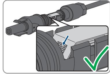
4. If the stranded wire is not visible in the chamber, the cable is not correctly inserted and the connector must be reassembled. To do this, the cable must be removed from the connector.
