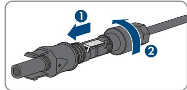
5. Push the swivel nut up to the thread and tighten (torque: 2 Nm).
