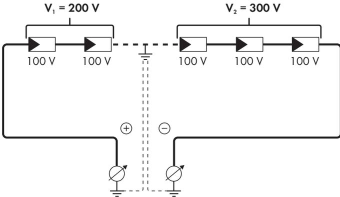
**Test by Measuring the Insulation Resistance**
