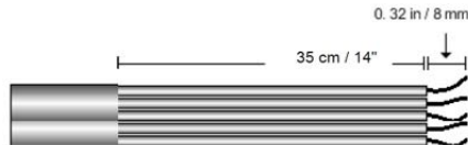
Figure 33: Insulation stripping – AC
