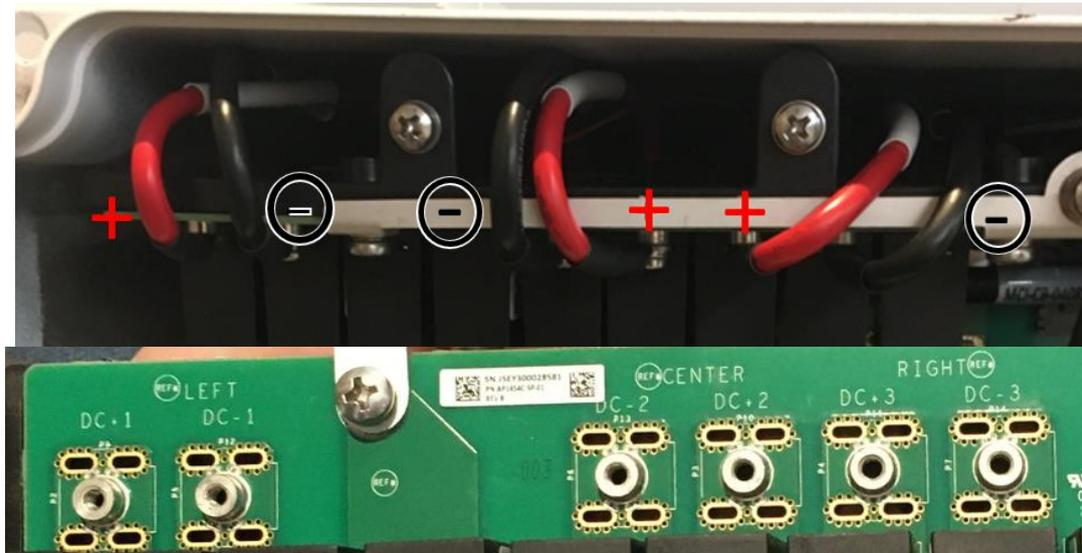
Figure 18: keep correct polarity
