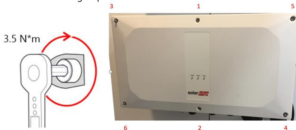
Figure 19: screw tightening sequence
