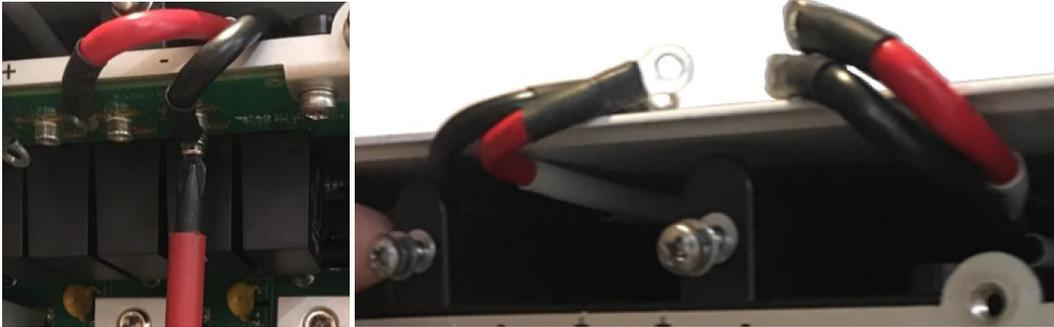
Figure 6: remove 6 screws
