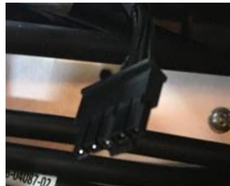
Figure 7: disconnect NTC cable
